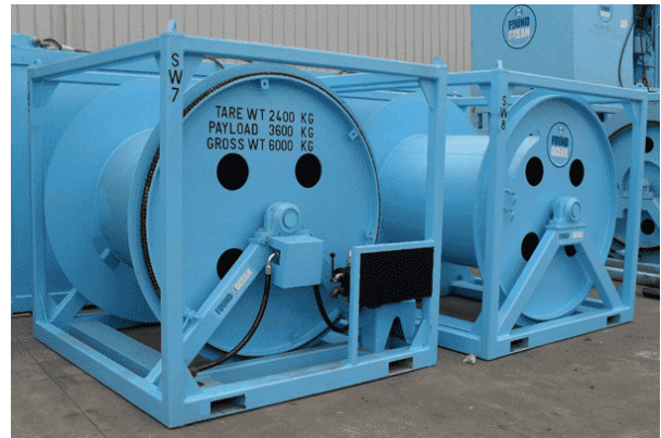
Hose storage reel prior to hose being attached.
