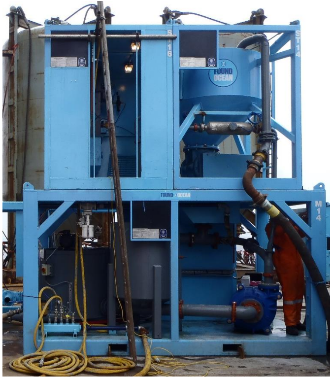
Assembled – Mixer and Surge Tank
