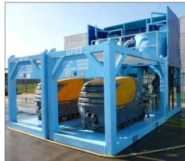
2 nos. Grout Pumps in their offshore lifting frames.
