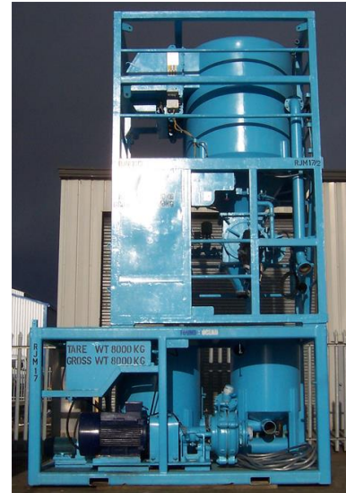
Assembled – Mixer and Surge Tank
