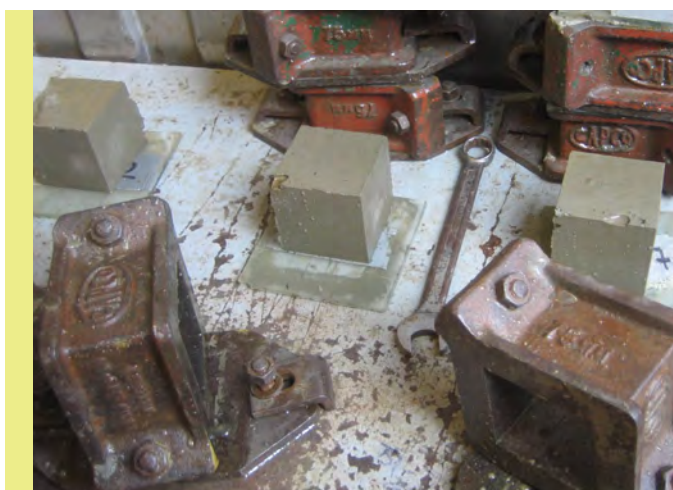
(above) Cubes being demoulded ready for testing
