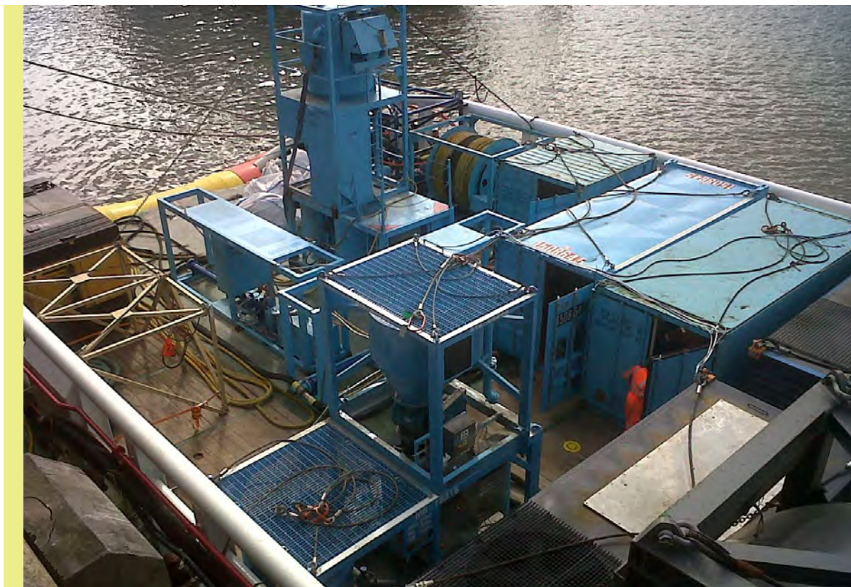
FoundOcean RJM16 grouting spread onboard the Else-Marie
