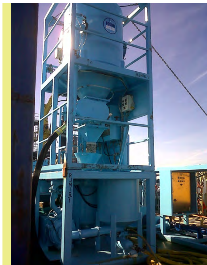
FoundOcean's unique Recirculating Jet Mixer (RJM) grouting spread
