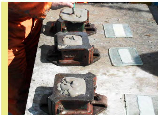
(above) A FoundOcean lab technician takes grout samples and manufactures cubes for testing
