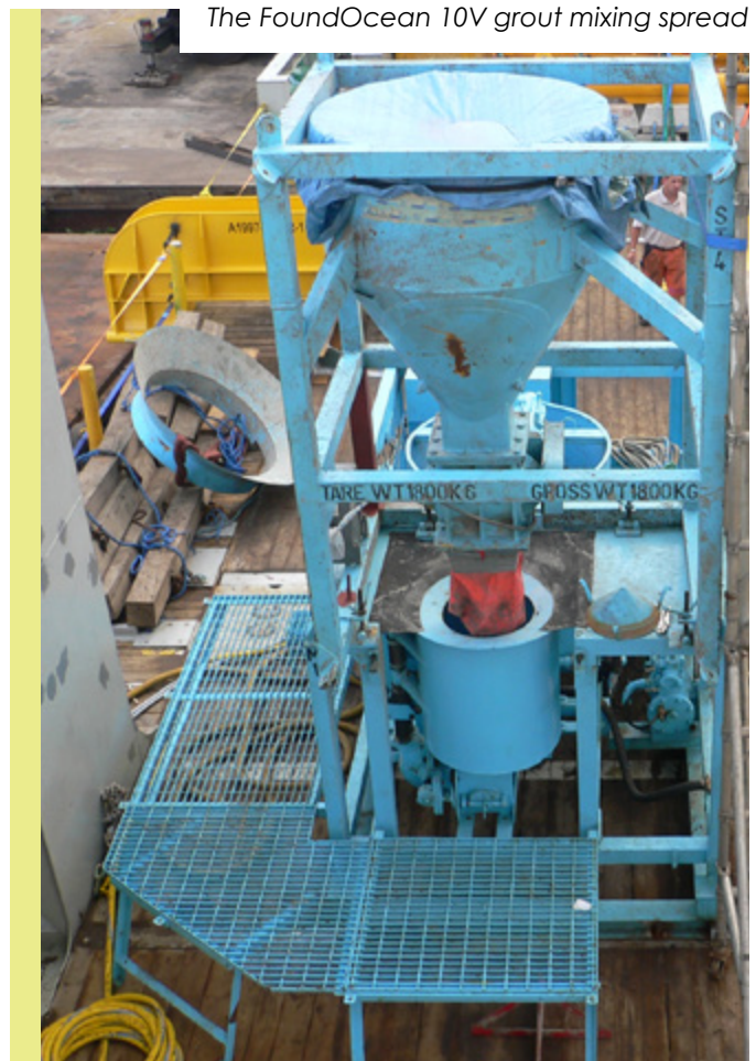
The FoundOcean 10V grout mixing spread
