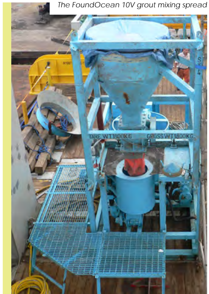
The FoundOcean 10V grout mixing spread
