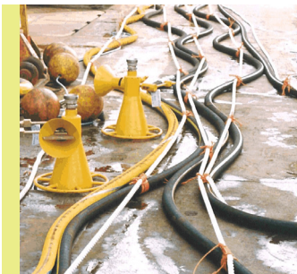
Female connectors and hoses laid out on board
