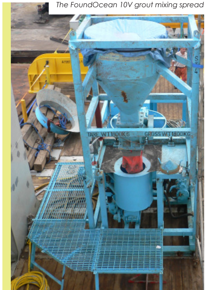
The FoundOcean 10V grout mixing spread
